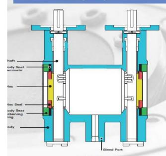
Two standard valves combined into one integral cast body. This eliminates the need for extra joints, gaskets and bolting which in turn reduces potential leak paths. Each disc is independently operated thus providing true double isolation.
