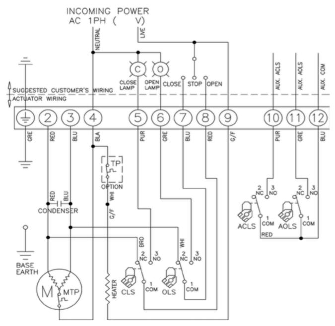
CLS : CLOSE LIMIT SWITCH (250VAC 3A) OLS : OPEN LIMIT SWITCH (250VAC 3A) ACLS : AUX. CLOSE LIMIT SWITCH (250VAC 3A) AOLS : AUX. OPEN LIMIT SWITCH (250VAC 3A) TP : THERMAL PROTECTOR (250VAC 15A OPTION) \*EACH ACTUATOR SHOULD BE POWERED THR-OUGH ITS OWN INDIVIDUAL SWITCH OR RELAY CONTACTS TO PREVENT CROSS FEED BETWEEN TWO OR MORE ACTUATORS.
